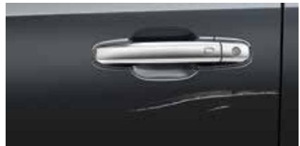
1 dent or 2 scratches (more than 4”) per panel
